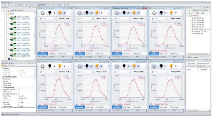
8 Channel Ethernet Network spectrometer for simultaneous tungsten spectral measurement and multi-windows simultaneous analysis with one PC
