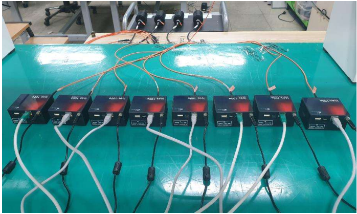
8 Channel Ethernet Network spectrometer for simultaneous tungsten spectral measurement and multi-windows simultaneous analysis with one PC
