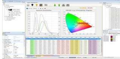
Produced LED wafer-specific light characteristics spread analysis results
