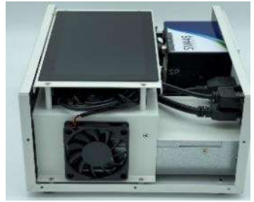
2 Example of a channel embedded OES system and built-in high-resolution spectrometer specifications
