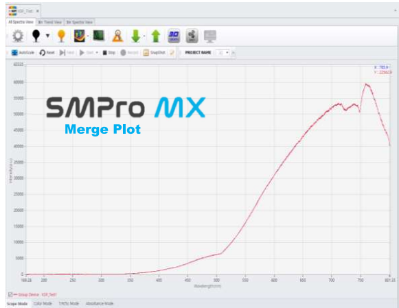
Outputs spectroscopy spectrum from different wavelength band spectrometers like a single spectrometer (High resolution 350 – 850 nm Merge tungsten spectrum)
